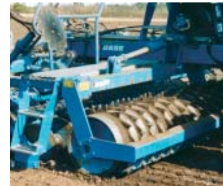
Zahnpackerwalze (Ø 66 cm) Toothed packer roller GZW (Ø 66 cm) Rouleau packer (Ø 66 cm)
