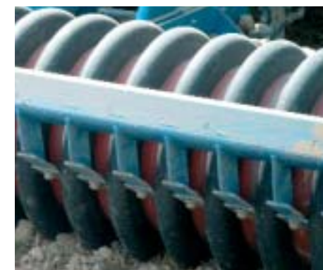
Rillenpackerwalze (Ø 58 cm) Wedge ring roller RIPA (Ø 58 cm) Rouleau sillonneur (Ø 58 cm)
