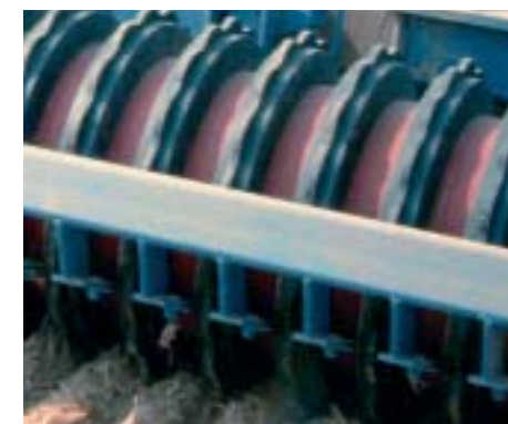
Mulchrillenpackerwalze (Ø 60 cm) Mulch wedge ring roller RIPA M (Ø 60 cm) Rouleau mulch sillonneur (Ø 60 cm)
